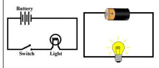
These are complete circuits - they have a battery (cell) and a component (bulb). The wires are placed in the right places of the battery for the circuit to work.
